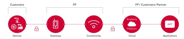
IoT closes the gap between the real and virtual (digital world) – IoT networks sensors and actuators with the cloud servers of providers or customers.
